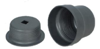
Revata Engineering's Pressed Steel Thread Protectors are designed & manufactured to protect the API Drill pipes, Drill Collars connections and tubing made as per API 5D, 7 & 5CT respectively.
